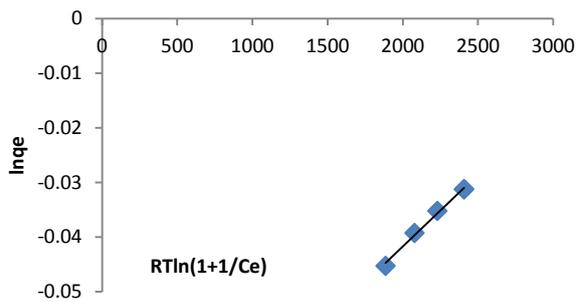
Fig.6 (a): Dubinin Raduskevich plot for adsorption of Cr(VI)
