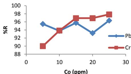
**Fig. 3(b): Effect of initial concentration on adsorption of Cr(VI) from binary solution (Adsorbent dose -1 g, contact time - 60 min, conc Pb(II) -20 ppm)**
