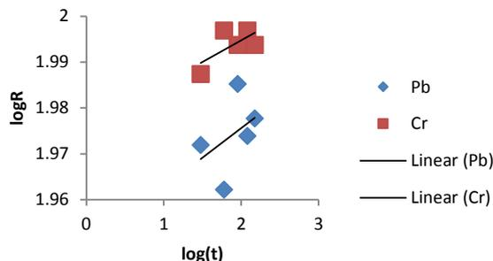
Fig. 9: The intraparticle diffusion kinetic model plot
