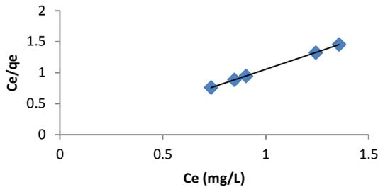
Fig. 4(b): Langmuir plot for adsorption of Pb(II) from the binary solution
