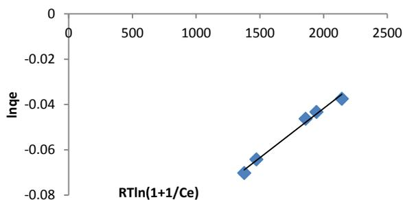
Fig. 6(b): Dubinin Raduskevich plot for adsorption of Pb(II)
