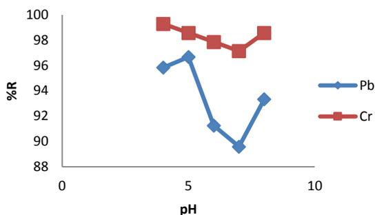
**Fig. 2: Effect of pH on the adsorption of Cr and Pb from a binary mixture**
