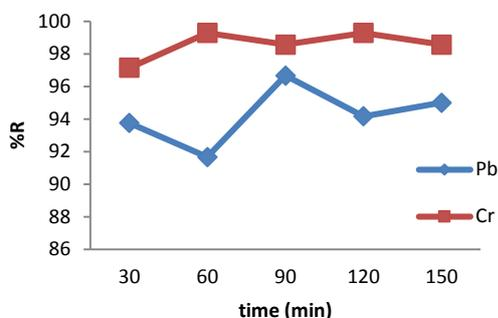
**Fig. 1: Effect of contact time on adsorption of Cr(VI) and Pb(II) from a binary solution**
