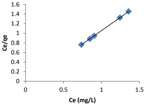
Fig. 4(a): Langmuir plot for adsorption of Cr(VI) from the binary solution
