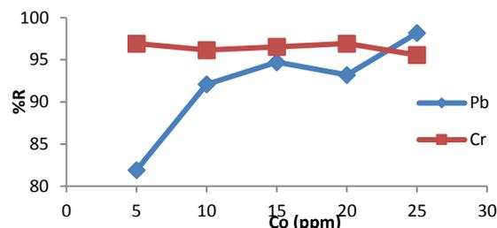
**Fig. 3(a): Effect of initial concentration on adsorption of Pb(II) from binary solution (Adsorbent dose -1 g, contact time -60 min, conc. Cr(VI) -20 ppm)**
